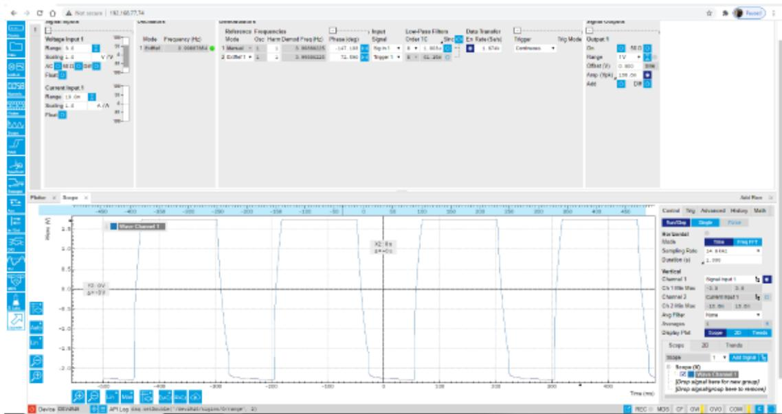
3. When you increase the chopping frequency, the voltage output drops as shown in a few examples below.
